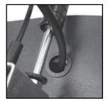
Insert Cable Connector Labeled SWITCH Through Bushing
