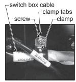
Secure Switch Box Cable Clamp
