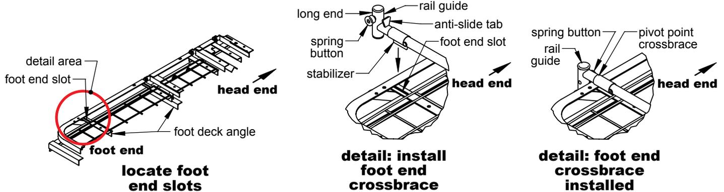
1. Locate the two foot deck angle slots on either side of the bed closest to the bed's foot end, shown in above left picture.
