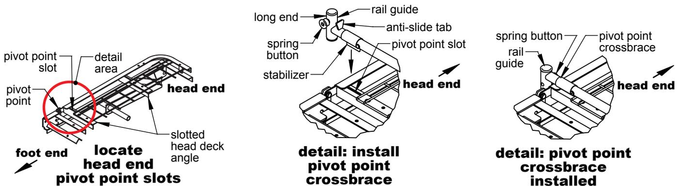
1. Locate the two head deck angle slots on either side of the bed closest to the head end pivot point, shown in above left picture.
