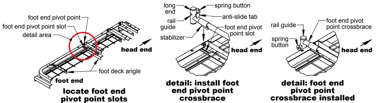
1. Locate the two foot deck angle slots on either side of the bed closest to the bed's foot end pivot point, shown in above left picture.
