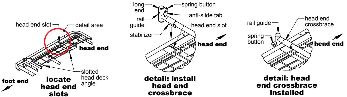
1. Locate the two head deck angle slots on either side of the bed closest to the bed's head end, shown in above left picture.
