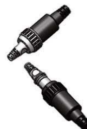
DETAIL B: ENSURE LOCK END CAPS ARE SCREWED ON SECURELY
