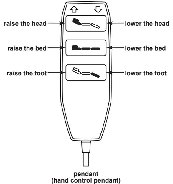
If any of the pendant functions do not work as expected, recheck all electrical connections to ensure all cables are seated properly within the motors and the control box, then retry the pendant function that did not work.
