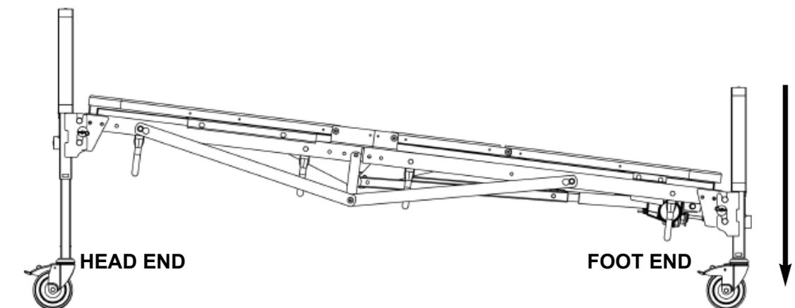
1. Raise the bed platform to its highest height. Disengage the HI / LO drive shaft by compressing the spring fitting at the head end and removing it from the head gear shaft and foot HI / LO motor: perform step 3 on page 15.
