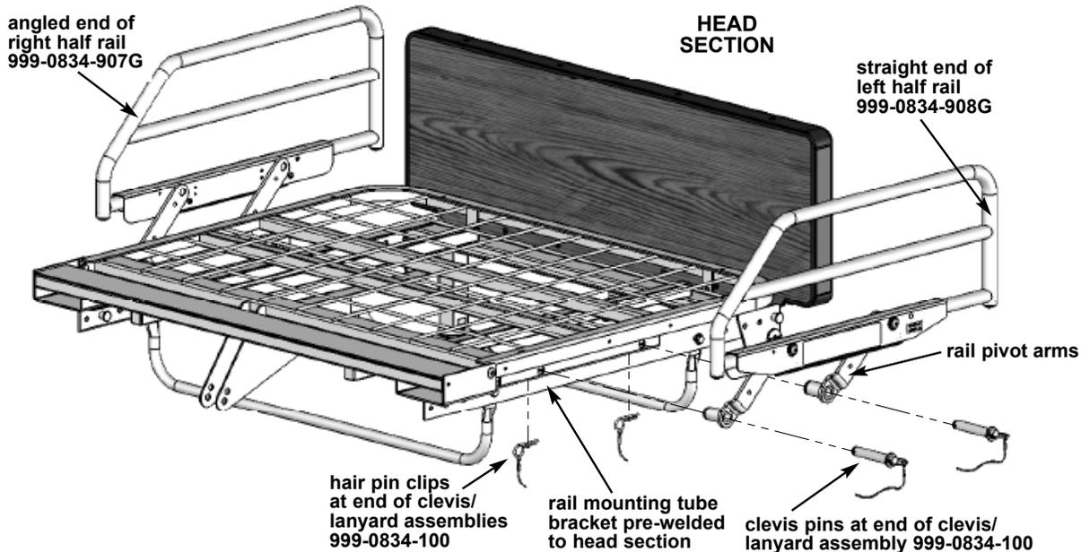
1. Align the rails so that the pivot arms face inward toward the bed and the straight ends of the rails face the head end as shown above.
