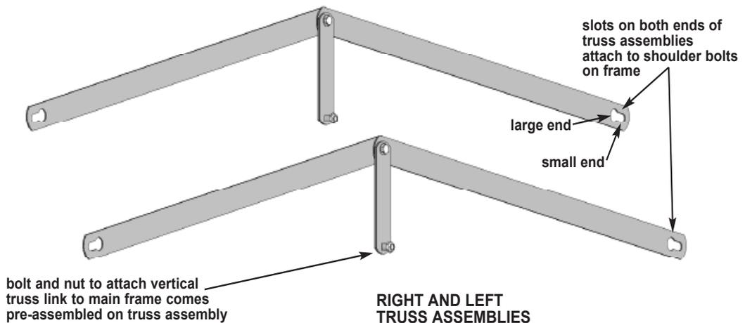
The two truss assemblies, shown above, span the decks and give them more stability, much like the trusses on a bridge. The trusses attach to the main frame via welded shoulder bolts on either side of the head and foot sections.
