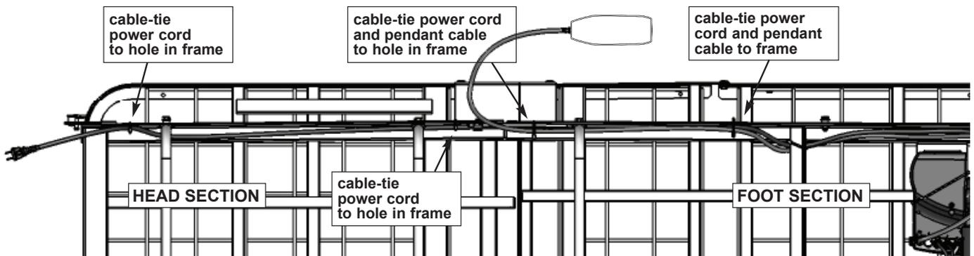
The head section of the bed does not come with any cable routing. The power cord and pendant cables will be coiled and cable-tied to the foot section in packaging. To route the power cord and pendant cable:
