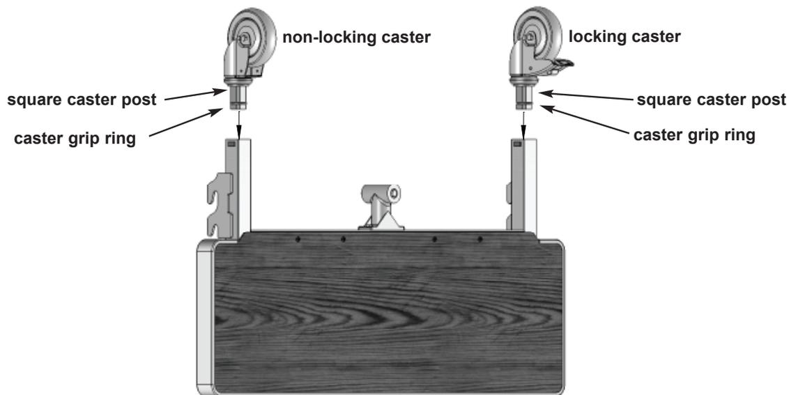
1. To install the casters in the bed end legs, insert the square caster posts directly into the bottoms of the legs, centering the caster grip rings in the legs as shown above.
