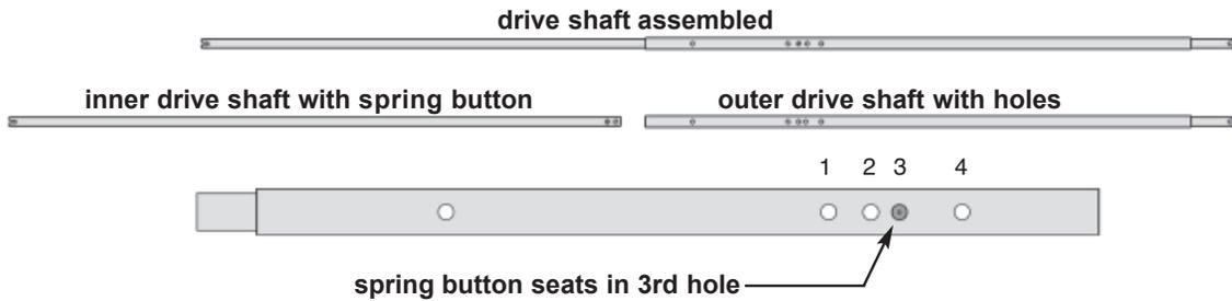
1. Lay the drive shaft parts on a flat surface so that the inner shaft is to your left and the outer shaft is to your right with the spring button end of the inner shaft facing the holed end of the outer shaft as shown above. The outer shaft also has a small spring-loaded inner shaft on the opposite end for ease of installation.
