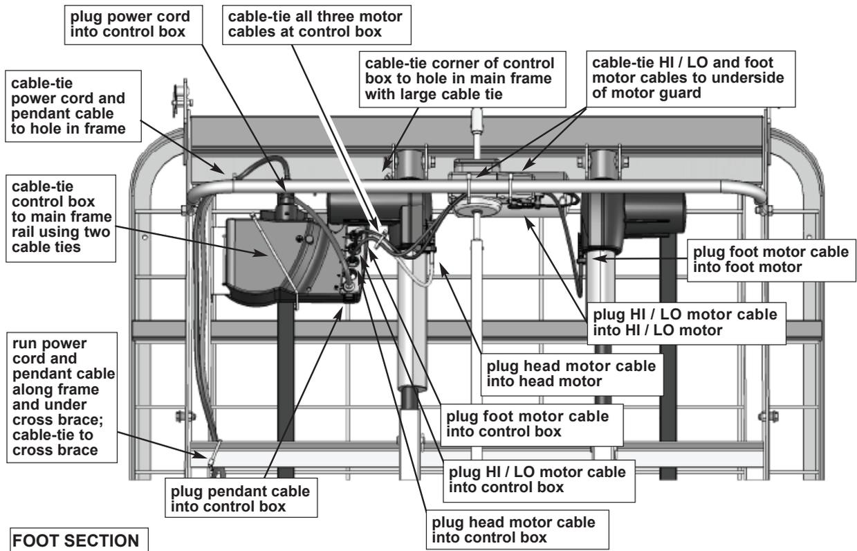
1. Cabling: The cables, shown above, will be installed at the factory on the foot section, as well as the control box, foot motor, HI / LO motor, and head motor. If you ever need to replace an electrical component or cabling, follow the diagram above.
