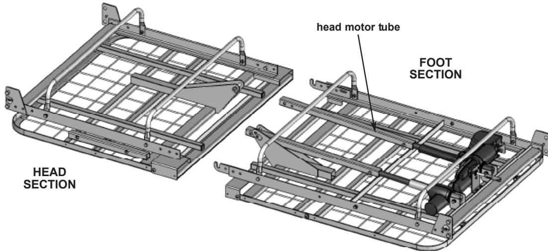
1. Lay the bed's foot section (with motors and junction box) upside down, flat on the floor, as shown above. Do the same with the head section close by.
