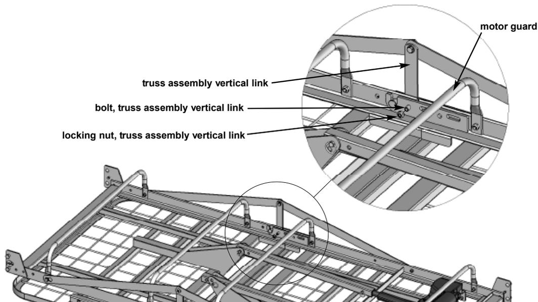
5. Attach the truss assembly vertical link to the main frame. Remove the nut from the bolt at the end of the vertical link as shown above. From the outside of the main frame, insert the bolt (with link) through the central hole. From the inside of the frame, secure the bolt using the same locking nut you removed earlier. Tighten both the bolt and the nut using two  $\frac{9}{16}$ " wrenches. Repeat for other side.
