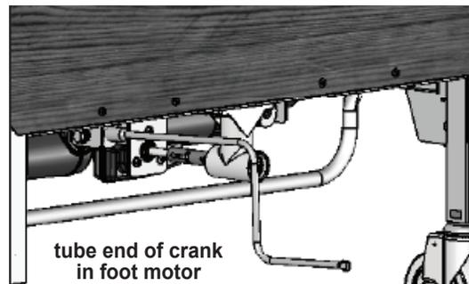
To lower the bed platform with the emergency crank, insert the crank's flat end into the HI / LO motor shaft slot as shown at above left and turn it counterclockwise.
