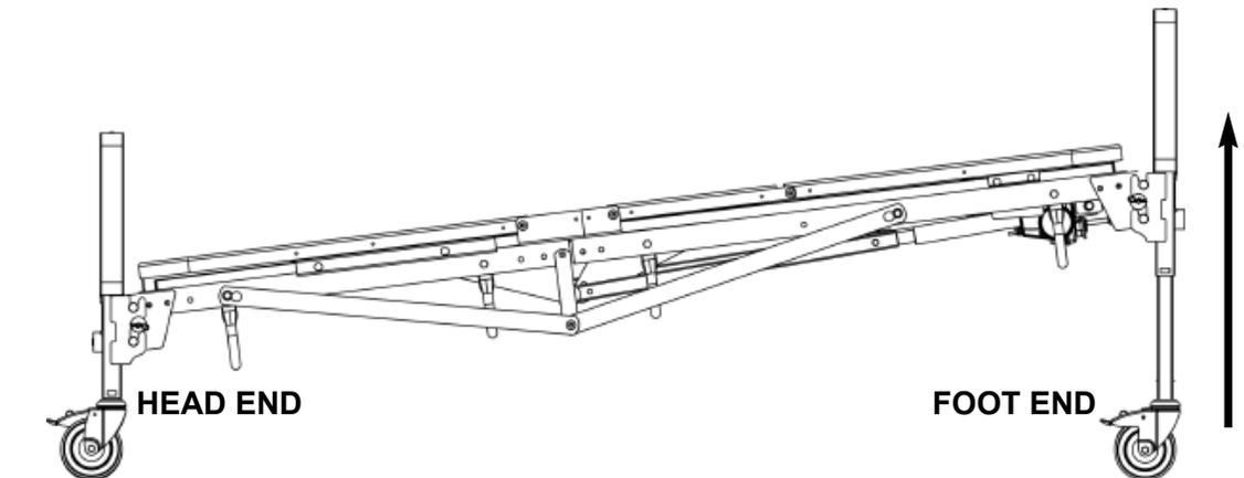
1. Lower the bed platform to its lowest height. Disengage the HI / LO drive shaft by compressing the spring fitting at the head end and removing it from the head gear shaft and foot HI / LO motor: perform step 3 on page 15.
