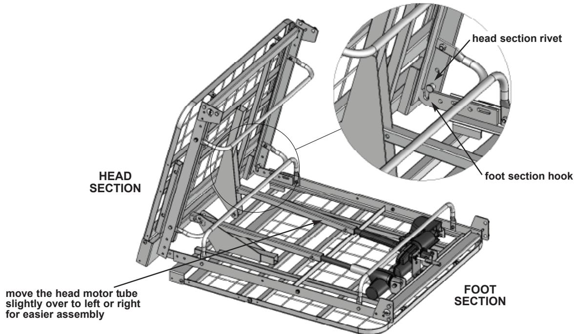
2. Move the head motor tube slightly over to the right or left to get it out of the way. Using two people, lift the head section so that it stands perpendicular to the foot section as shown above. Lift the head section and align the two rivets (on either side of the inside frame) with the two hooks in the foot section frame, as shown above. Lower and slowly maneuver the head deck so that the rivets seat in the hooks.
