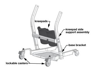
5. Insert the kneepad side support assembly into the base brackets as shown above. The kneepads and arm curvature should be facing away from the lockable casters.
