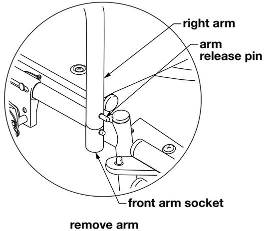
**⚠ WARNING:** Ensure arm release is locked in place before occupying or operating wheelchair.
