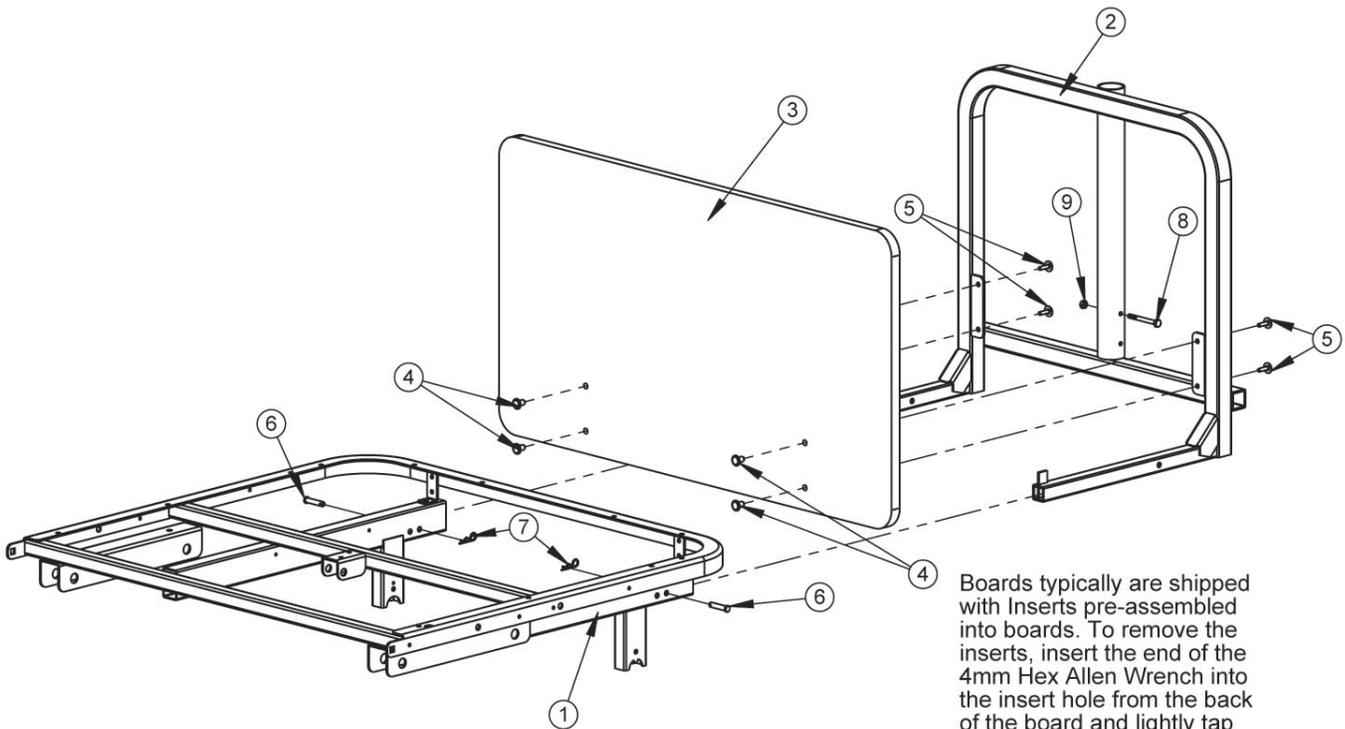
Boards typically are shipped with Inserts pre-assembled into boards. To remove the inserts, insert the end of the 4mm Hex Allen Wrench into the insert hole from the back of the board and lightly tap with a hammer.
