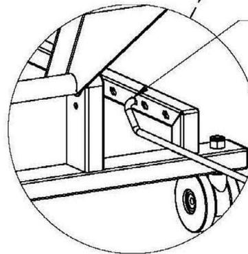
TO LOCK FLAT TAB INTO CARRIAGE RAIL, TURN TAB IN SIDE HOLE UNTIL WALLSAVER RESTS ON CROSSBRACE
