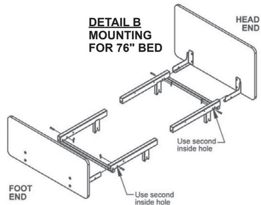
**NOTE: To order a new Headboard Panel Mounting Kit, use Part # 999-0822-000. Kit includes right and left Mounting Brackets, 8 Socket Head Cap Screws, 4 Clevis Pins, 4 Hair Pin Clips, and 1 Hex Key. Headboard and Footboard kits are sold separately.**
