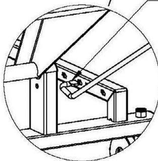
INSERT FLAT TAB SO THAT IT IS PARALLEL WITH CASTER CARRIAGE RAIL SLOT
