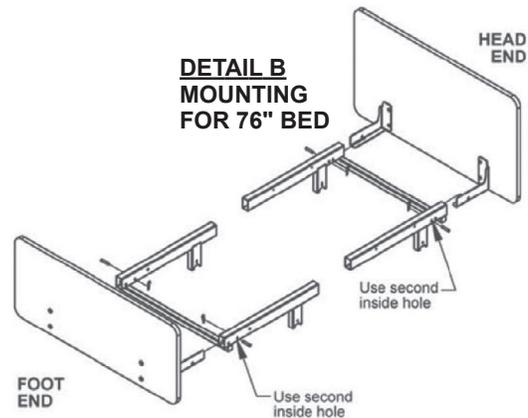
**NOTE: To order a new Footboard Panel Mounting Kit, use part # 999-0822-000. Kit includes right and left Mounting Brackets, 8 Socket Head Cap Screws, 4 Clevis Pins, 4 Hair Pin Clips, and 1 Hex Key. Headboard and Footboard kits are sold separately.**
