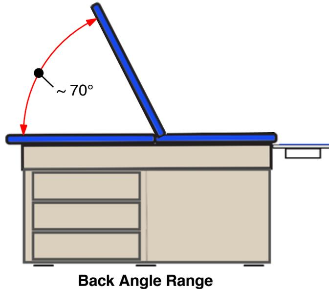
The exam table features a limited back angle of  $\sim 70^\circ$  to accommodate heavier occupants comfortably, as shown above.
