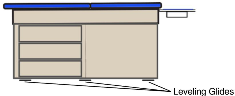
1. Locate Leveling Glides on Bottom of exam table base, shown above (six total).
