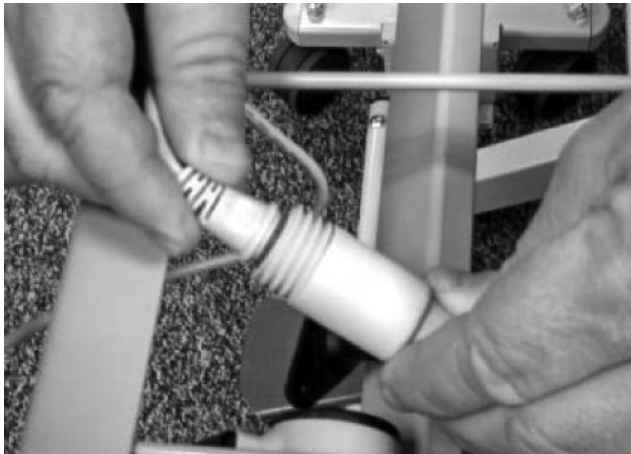
Improper Connection (not completely seated)
