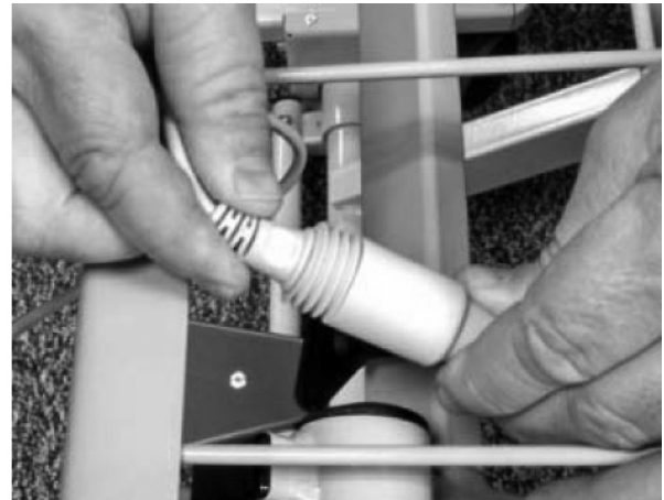
Proper Connection (completely seated)
