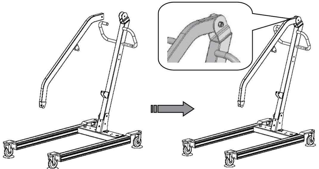
7. Attach the control box hanging bracket to the mast. Tighten the nuts.
