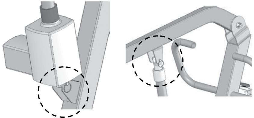
10. Attach the actuator top to the boom bracket and insert retainer pin. Insert retaining ring through retainer pin hole to secure actuator top to boom bracket.
