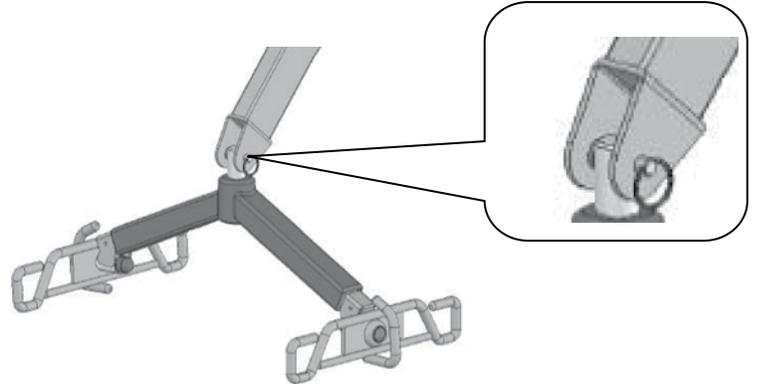
11. Attach the spreader bar bracket to the boom and insert retainer pin. Insert retaining ring through retainer pin to secure spreader bar to boom.
