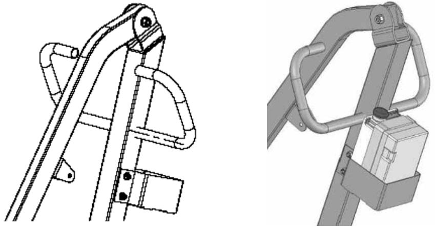
9. Attach the actuator bottom to the mast bracket and insert retainer pin. Insert retaining ring through retainer pin hole to secure actuator base to mast bracket.
