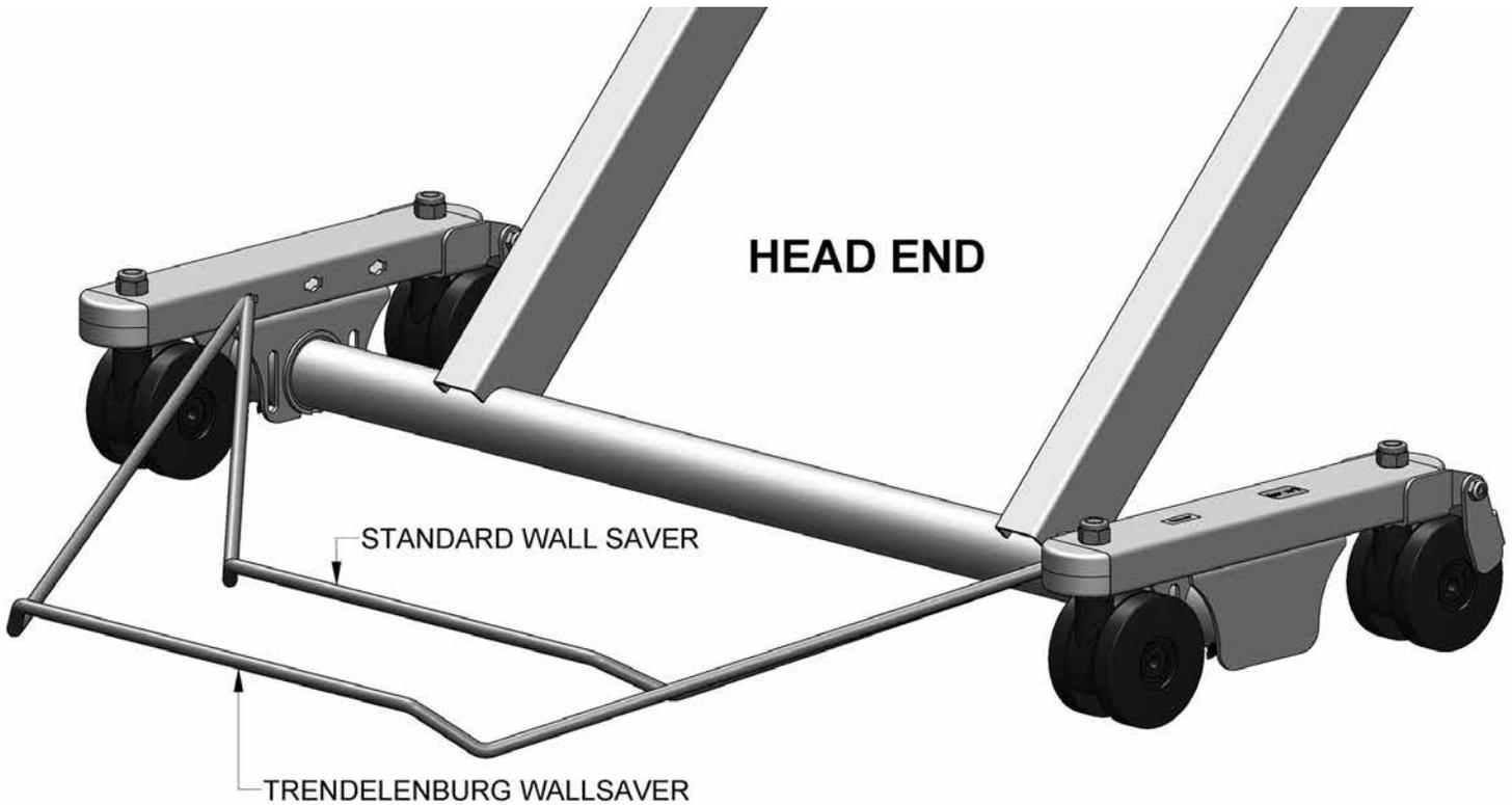
1. Position the Wireform Wallsaver ***with bent end facing upward*** and tab ends facing inward as shown above.
