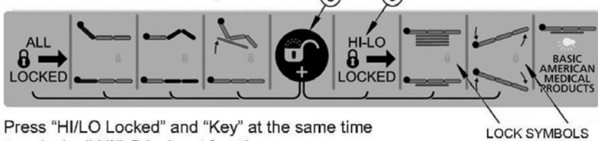
Press "HI/LO Locked" and "Key" at the same time to unlock all HI/LO lock out functions.
