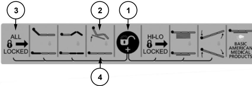
1. Ensure the Chair position on the Staff Control panel is not locked out (*orange lock icon*). To unlock, press Lock icon #1 and Chair icon button #2 (or "All Locked" button #3) simultaneously.
