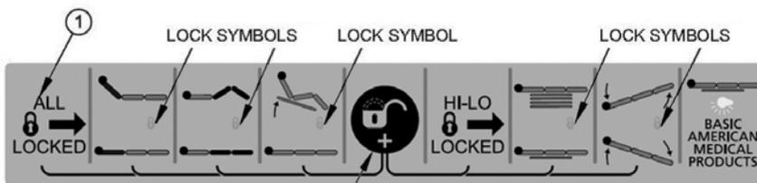
Press "All Locked" and "Key" at the same time to unlock all functions.
