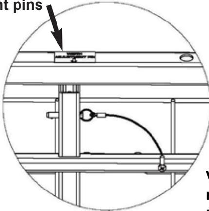
3. Stand at the side of the bed and place your hands near the detent pin labels (your hands must be this widely spaced) and hold the entire left or right side of the expandable deck (not the ends). Pull the deck out toward you to expand, or push the deck inward toward center to retract. On the underside, align the desired hole position on the deck insert tubes with the single hole in the end of the mainframe cross tubes (see below).
