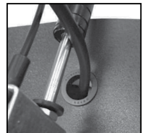
Insert Cable Connector Labeled SEAT Through Bushing
