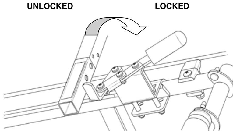
The Regency 5600 has two wheel locks — one on each rear wheel. To engage the wheel locks, push the levers forward until they lock into place, as shown above. To disengage, pull back on the levers until the wheels roll freely.
