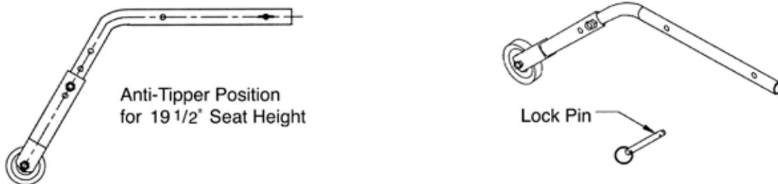
We recommend the use of anti-tippers at all times. The appropriate anti-tipper setting for your wheelchair's seat height is shown at above left.
