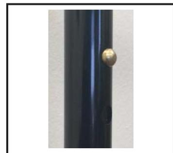
3. Slide the lower tube extension up or down until the snap button pushes through the adjustment hole completely at the correct height. You will hear a click. If you cannot see the push button completely, the cane height is NOT secure.
